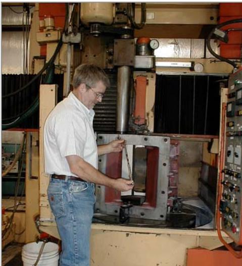
in diameter and the machine is capable of swinging parts as large as 76" in diameter. The unit is able to work up to a full 41" under the rail making our ability to handle large piece work quite unique.
